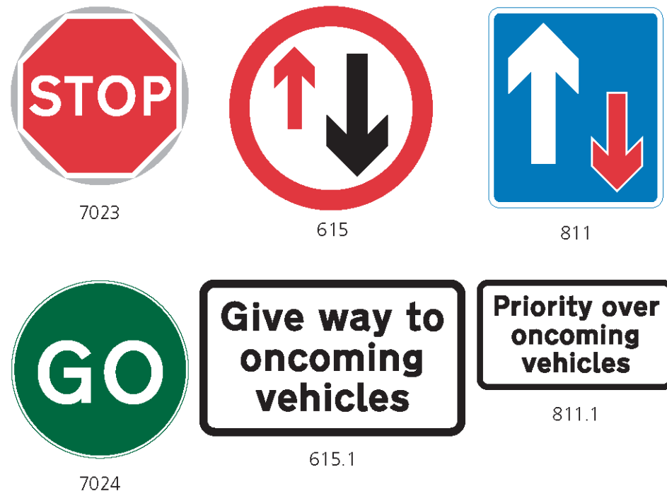
Figure 3.5: Manually Operated Stop/Go Signs and Priority Signs.
